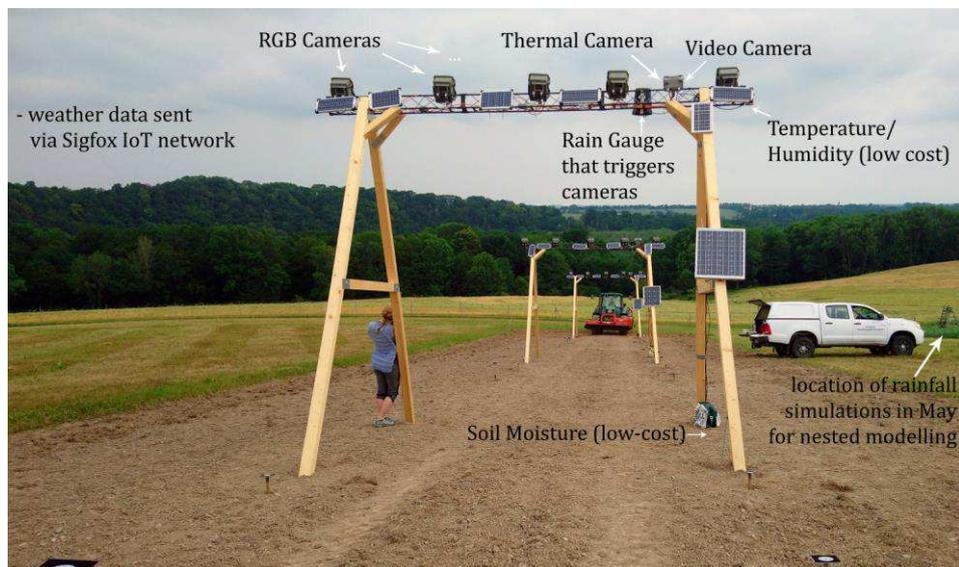
Figure 1: Hillslope setup to measure soil erosion during the rainfall event based on time-lapse SfM photogrammetry
