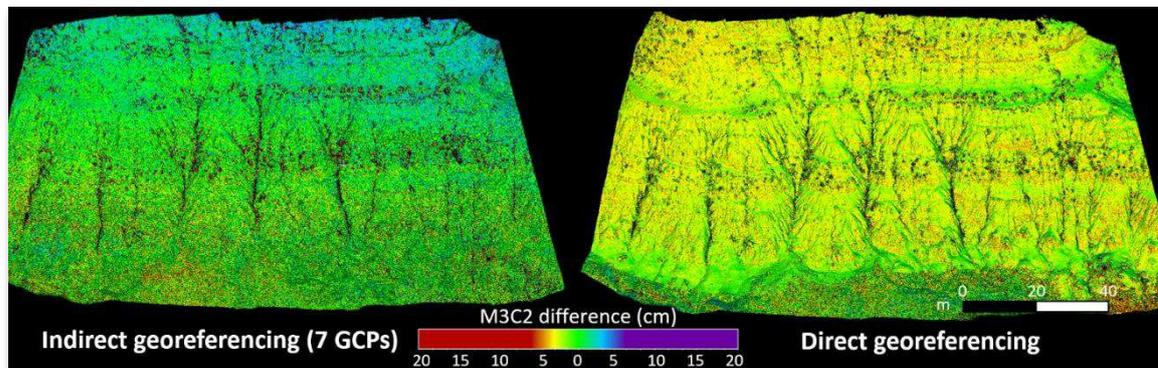
Figure 2. M3C2 difference between UAV datasets and ground-based LiDAR reference dataset. Left: indirect georeferencing with 7 GCPs (mean = 3 cm); Right: direct georeferencing (no GCPs) using RTK-UAV (mean = 4 cm).
