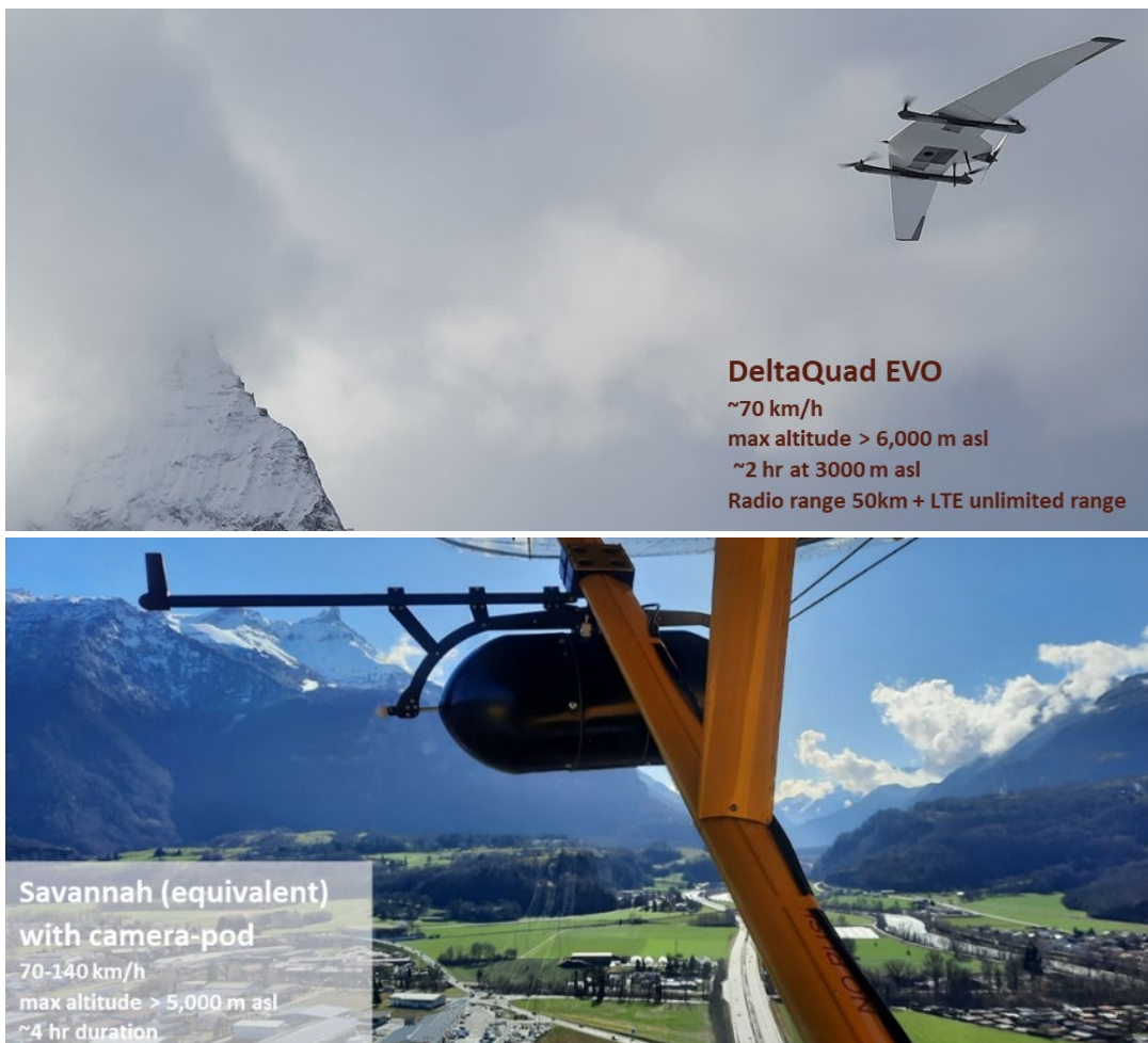
Figure 1: DeltaQuad EVO autonomous VTOL drone (above) and the dual-camera pod attached to a plane (below)
